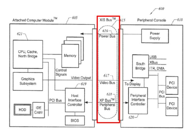
Annotated Figure 6 above shows a block diagram of a computer system using an interface. Ex. 1001, 15:15–16. As shown, computer system 600 includes attached computer module (ACM) 605 and peripheral console 610. *Id.* at 15:16–18. ACM 605 and peripheral console 610 are interfaced through exchange interface system (XIS) bus 615. *Id.* at 15:23–24. XIS bus 615 includes power bus 616, video bus 617 and peripheral bus (XPBus) 618, which is also referred to as an interface channel. *Id.* at 15:24–27.
