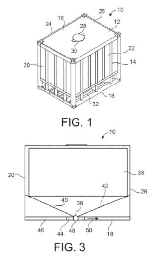
includes inlet 28 for receiving proppant and outlet 36 through which proppant can be discharged. Gate 44 can be actuated to cover or uncover outlet 36, thereby preventing or permitting the discharge of proppant. Pin 48 protrudes from gate 44.
