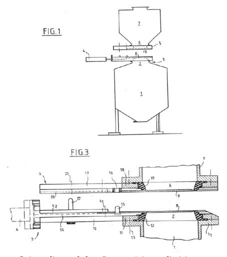
It is undisputed that Constantin's non-limiting example, standing alone, discloses the opposite of the '341 configuration. More specifically, Constantin's example includes an actuator having the pin (Constantin's "actuating device" 4 having "stud" 15) and a gate having the receptacle (Constantin's "shutter blade" 9 with "orifice" 16).
