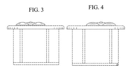
Figures 3 and 4, above left and right, respectively, each show side views of the claimed switch design along shorter edges of the switch; Figure 3 showing the switch from one end and Figure 4 showing the switch from the opposite end.
