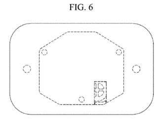
Figure 6, above, shows a bottom view of the claimed switch design.
