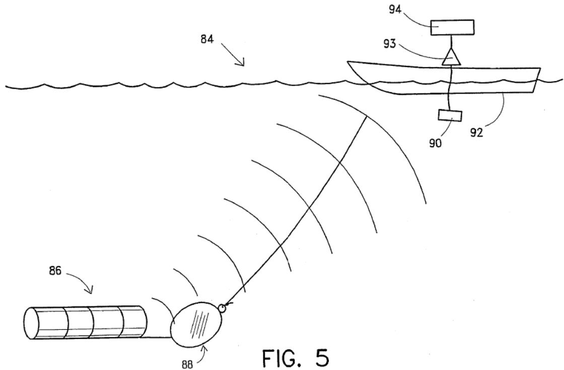
Figure 5 is a diagrammatic view of Langer's fish detection system. Ex. 1006, 3:57. In Figure 5, underwater detection system 84 includes sensor 86 that is coupled to lure 88. *Id.* at 12:57–58. Sensor 86 transmits signals
