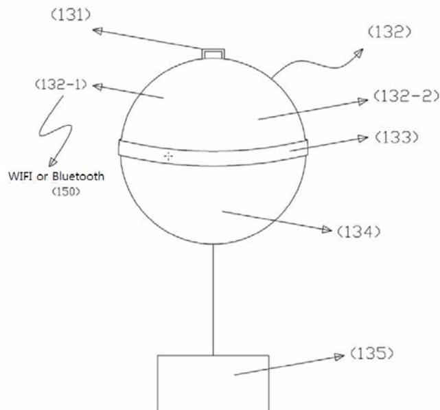
Figure 7 is a block diagram showing the front of buoy-type fish finder 130 in more detail. Ex. 1004, 6. Buoy type fish finder 130 includes rope hook 131, fish finder 132, patch antenna 132-1, battery 132-2, buoy 133, control module 134, and ultrasonic sensor 135. *Id.* at 8–9.
