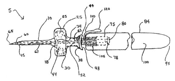
The sole Figure from Lynn, above, depicts vascular access system 5 including a needle protective device (needle receptacle 84) for receiving spring biased needle 60. According to Lynn, when a user depresses button 120, spring 105 is released from a compressed state retracting needle 60 into receptacle chamber 100. *Id.* at 7:15–26.
