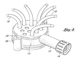
Figure 4 is a perspective view of Cooper's sprinkler. *Id.* at 2:8–9, 3:20–22. As shown in Figure 4, the "tubes may be bent . . . by the user into any desired curve." *Id.* at 3:20–22.
