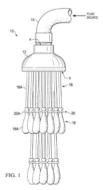
Figure 1 is a simplified diagram illustrating an example embodiment of system 10 for filling containers with fluids. *Id.* at 2:36–37. As shown in Figure 1, system 10 includes housing 12 removably attached to hose 14 at
