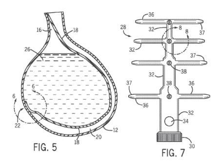
Figure 5 is a cross-sectional view showing Saggio's tie-less water balloon filled with water. Id. ¶ 13. Figure 7 is a front elevation view of a multi-balloon filling assembly. Id. ¶ 15.
