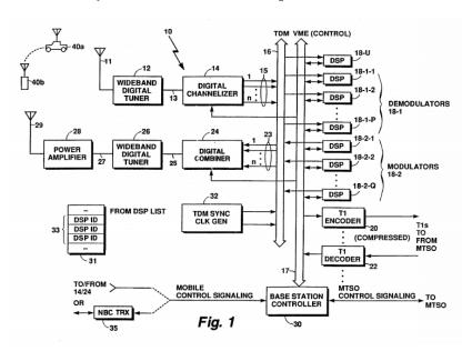
'480 patent, Fig. 1. Both Figures 1 depict the wideband digital basestation 10 communicating with mobile terminals 40 via radio frequency (RF) signals. Also, Figure 2 of the '408 patent and Figure 2 of the '480 patent show the same routing of data on and off the TDM bus to the digital signal processors.
