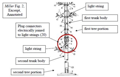
Petitioner's annotated version of Miller's Figure 2 depicts an artificial tree with first and second light strings, trunk bodies, and tree portions. The electrical connector between tree portions is a loose, plug-and-socket connection housed within the hollow trunk bodies. *See* Ex. 1006, 2:19–68 (describing a "main double conductor wire 22 extending lengthwise of trunk").
