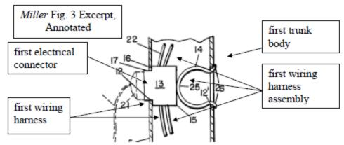
Petitioner's annotated, excerpted Figure 3 of Miller depicts a cross-sectional view of an artificial tree, showing the trunk and details of a wiring harness. Pet. I 49.
