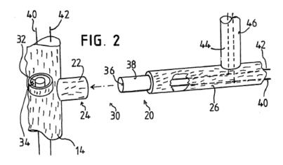
Figure 2 of Otto is a perspective view of a branch having a plug being connected into a socket on a trunk portion. Otto describes how trunk and branch components electrically and mechanically connect using coaxial connections, which makes it "easy to put the connecting areas together, and the branches and trunk elements may be rotated relative to one another even in the assembled state, so that any desired configuration of the Christmas tree is achieved." Ex. 1008, 18:23–27.
