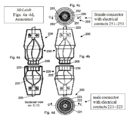
Figures 4a–4d of McLeish depict multiple views of the McLeish coaxial connector, including views of the male and female connector ends, a cross section view, and a perspective view with the internal electrical components depicted in ghost form. Petitioner characterizes the combination as "combining prior art elements with each performing the same function it had been known to perform to yield what one would expect from such an arrangement." Pet. I 37.
