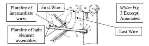
Petitioner's annotated, excerpted Figure 3 of Miller depicts a crosssectional view of an artificial tree with a branch extending therefrom, showing in dashed lines two lighting elements connected to a wiring harness on the trunk. Pet. I 54.
