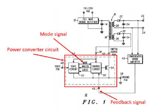
Figure 1 depicts power supply 10 using integrated power converter circuit 44. Power supply 10 is controlled by power converter circuit 44, which includes five pins: bias pin 36, ground pin 38, feedback pin 46, state pin 48,
