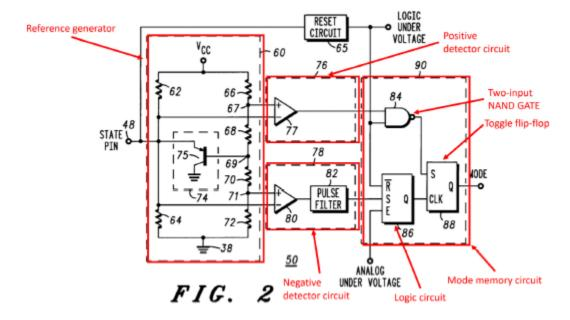
Figure 2 depicts an embodiment of the state circuit portion of power converter circuit 44. "The state circuit includes reference generator 60, which is a resistance network that creates threshold voltages for the comparators of the positive detector circuit 76 and negative detector circuit 78." Pet. 8 (citing Ex. 1001, 3:66–4:2). The Specification describes that the resistance network may generate reference voltages of 2.9 volts (at node 67)
