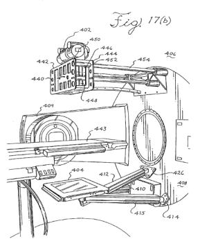
Specifically, Figure 17(b) above shows wall-mounted cone beam computerized tomography system 400 including an x-ray source, such as x-ray tube 402, and flat-panel imager 404 mounted on gantry 406. *Id.* at 19:41–43. X-ray tube 402 generates beam of x-rays 407 in a form of a cone
