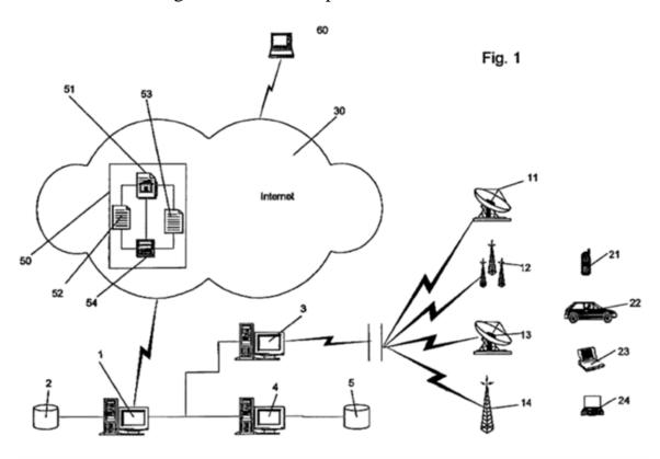
Figure 1 illustrates mobile platforms, including mobile telephone 21, car 22, laptop 23, and briefcase 24, and location tracking systems 11, 12, 13, 14 that communicate with communication subsystem 3 of location determination system 1. *Id.* at 3:31–32; 3:44–4:11.
